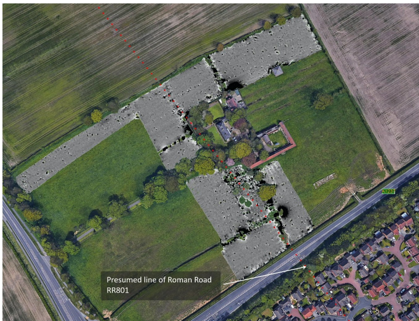
Fig 2, Plot of Gradiometer survey of land surrounding Ings House, Skelton, York, superimposed on Google Imagery
